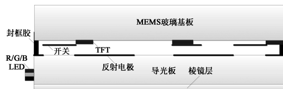
图 4 DMS 显示器件的典型的光学结构 Fig. 4 Typical optical structure of DMS display device
